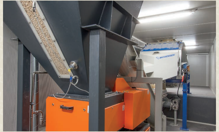
A screw connects the sizer to the weigher.
