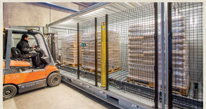
When the last container is full and contains three finished pallets, the wrapper stops. As soon as the pallet closest to the door has been collected, a photocell starts the roller conveyors, the two remaining pallets are moved forward, and the wrapper starts again. A fence and a light barrier provide the same security as for standard plants.
