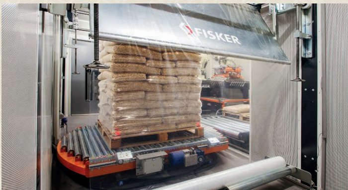
Fully automatic stretch film wrapper. Once the pallet has been wrapped, it is transported to the last container ready for collection.
