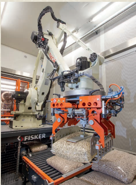
Palletising of sacks using a Nachi robot palletiser.
