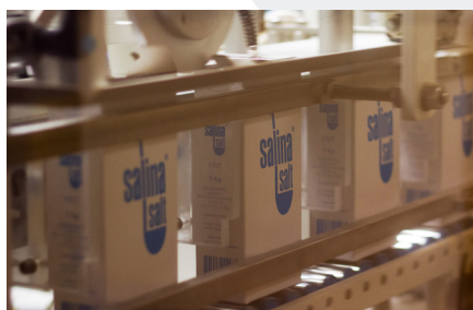
The new packaging line packs salt daily in boxes of 250, 500 and 800 grams as well as 1 kg.
